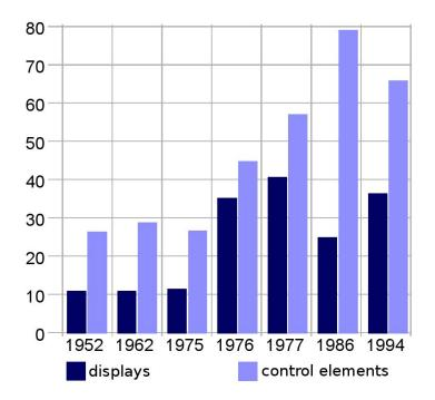
Figure 1: Increase of displays and control elements in BMW cars [2]
