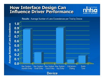
Figure 2: How interface design can influence driver performance [4]
