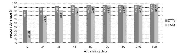
Figure 8: recognition rate for Dynamic Time Warping algorithm (DTW 3.3.2) and Hidden Markov Models (HMM 3.3.1) [2]
