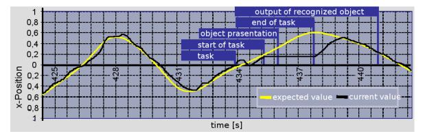
Figure 9: study schedule: while steering the user has to execute a second task, like tune radio to 93.3 MHz, and recognize an object.[2]
