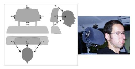
Figure 7: sensor arrangement for head gesture recognition: schematic diagram (left) and real installation with user(right) [2]
