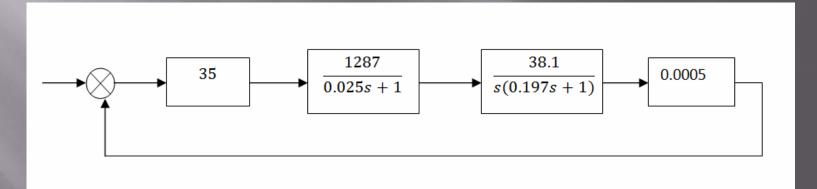
It is classical configuration of systems of such class with a negative feedback.
