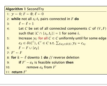
The reverse deletion step is not strictly necessary this way. It would also be sufficient to simply delete all unnecessary edges in any order.
