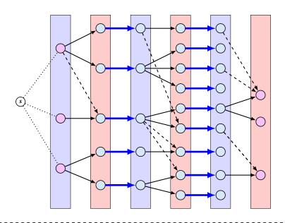
Every shortest alternating path is a path in this graph from a left free vertex to a right free vertex; find a maximal vertex disjoint set of path by a modified DFS
