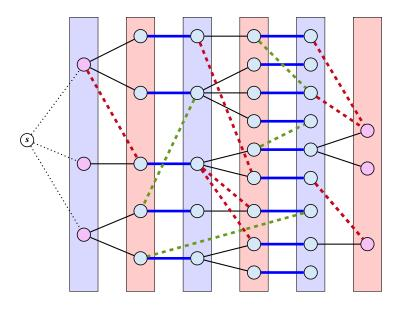
This fixes length of shortest alternating path; every shortest alternating path must visit layers from left to right (green edges are not helpful)
