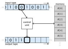
Note that in the picture on the right the tapes are one-directional, and that a READ- or WRITE-operation always advances its tape.
