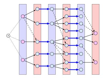
Every shortest alternating path is a path in this graph from a left free vertex to a right free vertex; find a maximal vertex disjoint set of path by a modified DFS
