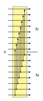
If we feed a bitonic 0-1 sequence S into the network on the right we obtain two bitonic sequences  $S_T$  and  $S_B$  s.t.
