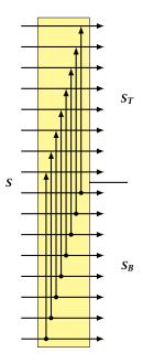
If we feed a bitonic 0-1 sequence S into the network on the right we obtain two bitonic sequences  $S_T$  and  $S_B$  s.t.
