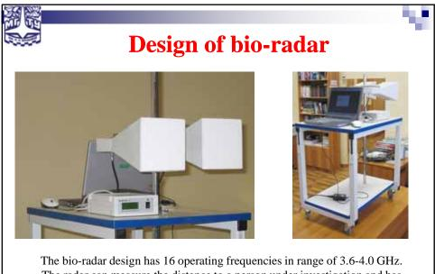
The bio-radar design has 16 operating frequencies in range of 3.6-4.0 GHz. The radar can measure the distance to a person under investigation and has improved abilities to filter noise and background reflections.
