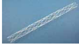
Igaki-Tamai biodegradable peripheral PLLA-based stent
