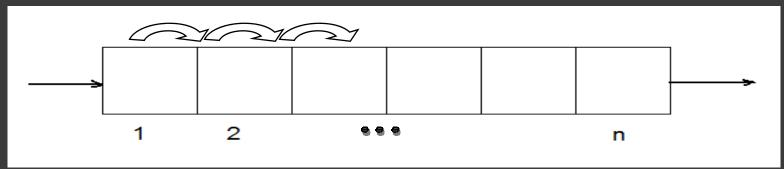
Incoming data is always stored in first cell of FIFO. After data is stored, shifting of data is performed. Because of this shifting, first inputted data would be always first to out.
