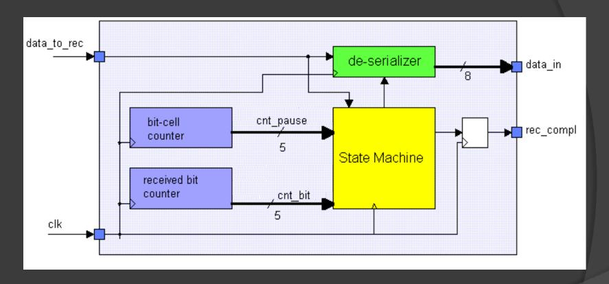
Receiver is used for receiving data from 1 bit input and to transform this data to 8 bit output.
