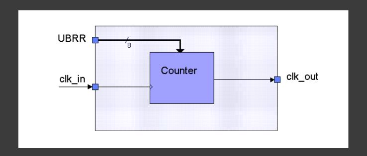
Baud rate generator is used for setting internal clock frequency and for changing transfer rate of UART.
