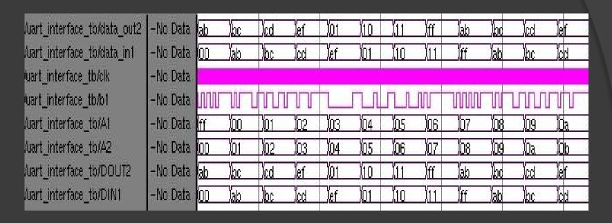
In this time 2 UART was connected to each other. First UART was transmitting data from 8x256 memory, and second UART was receiving incoming data and stored it in its empty memory.
