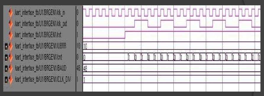
To make baud rate generator operate we need to activate it. This picture shows activation process. Low level on RST input starts UART. After activation low level on RST resets UART.
