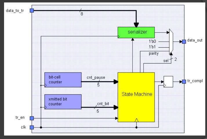
Transmitter is used to shift 8 bit data bit by bit to data bus.
