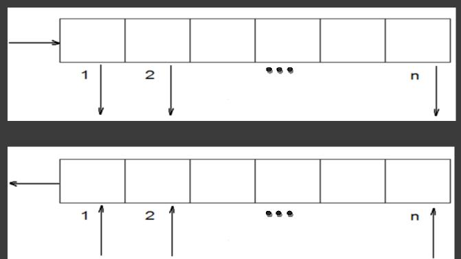
UART is based on shift register. There 2 registers – one in receiver and one in transmitter
