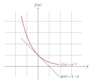
The inequality  $1 - x \le e^{-x}$  is derived by stopping the tayler-expansion of  $e^{-x}$  after the second term.
