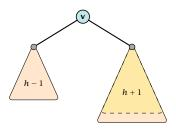
The right sub-tree of v has increased its height which results in a balance of -2 at v.
