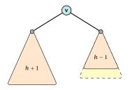
The right sub-tree of v has decreased its height which results in a balance of 2 at v.
