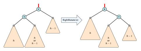
If the middle subtree has height h the whole tree has height h+2 as before the deletion. The iteration stops as the balance at the root is non-zero.
