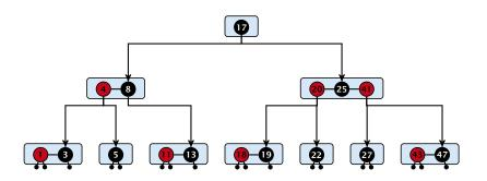
Re-attach the pointers to individual keys. A pointer that is between two keys is attached as a child of the red key. The incoming pointer, points to the black key.
