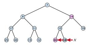
Note that an exchange can either be done by moving the data or by changing pointers. The latter method leads to an addressable priority queue.
