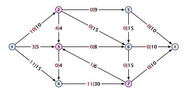
A node that has  $\sum_{e \in \text{out}(v)} f(e) < \sum_{e \in \text{into}(v)} f(e)$  is called an active node.
